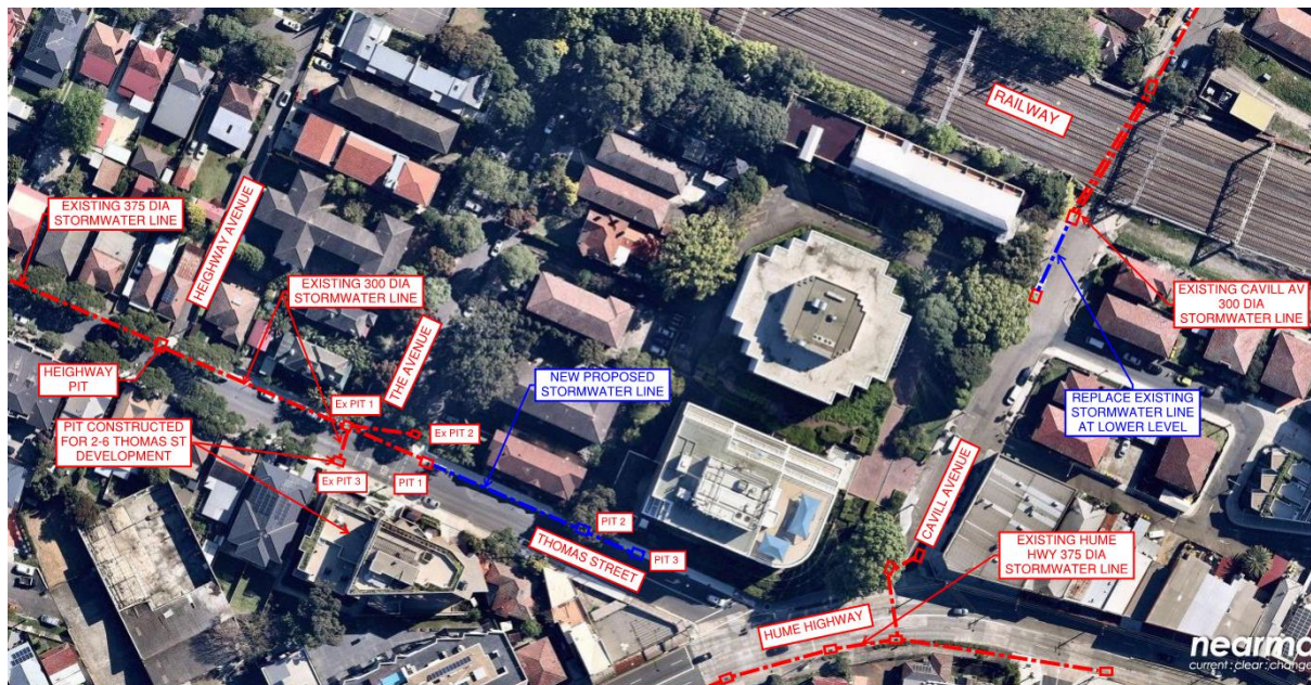
Figure 4 – Existing/Proposed Stormwater System
